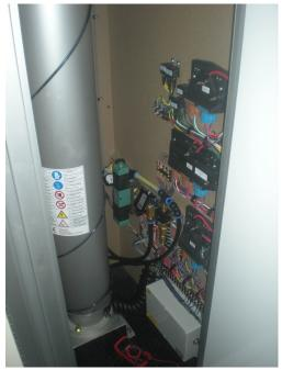
Figure 24. Antenna cylinder and cylinder stop sensor bracket in the Homeland Security Emergency Preparedness bus.
