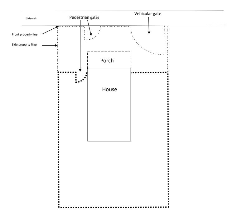
=5'-0" high, solid metal picket fence ===7'-0" high capped, wood vertical board fence
