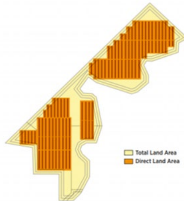
Example of total vs. direct land use in a ground-mount PV system
