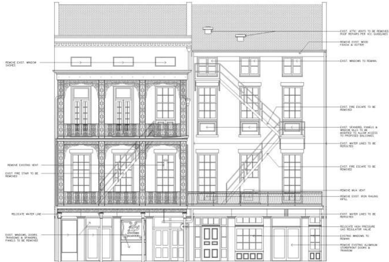
02 EXISTING IBERVILLE STREET ELEVATION A2.1 Scale: 1/4"=1'-0"
