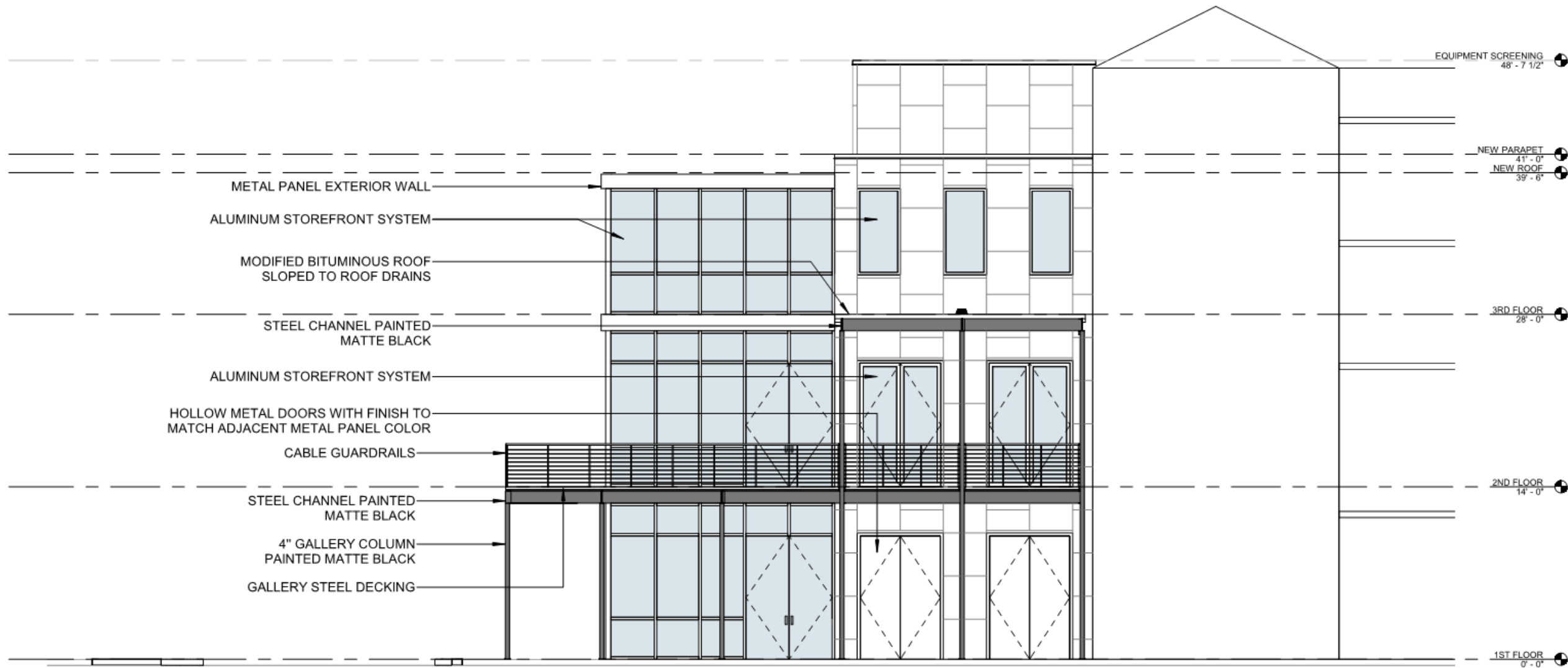
① DECATUR STREET ELEVATION 1/8" = 1'-0"
