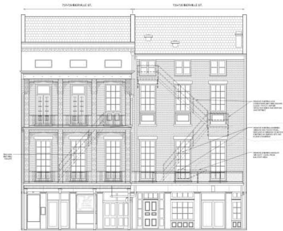
IBERVILLE ST. ELEVATION SCALE: 1/4" = 1'-0"
