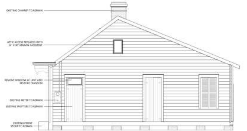
1 SOUTH ELEVATION PROPOSED 1/8" = 1'-0"
