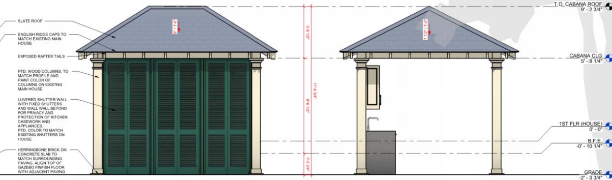
6 GAZEBO EXTERIOR ELEVATION - WEST 1/2" = 1'-0"
