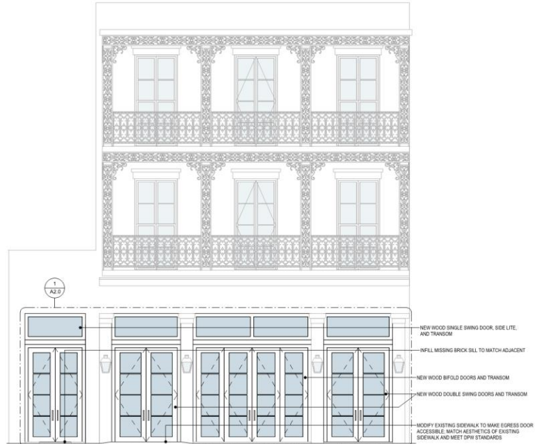
2 PROPOSED BOURBON STREET ELEVATION 1/4" = 1'-0"
