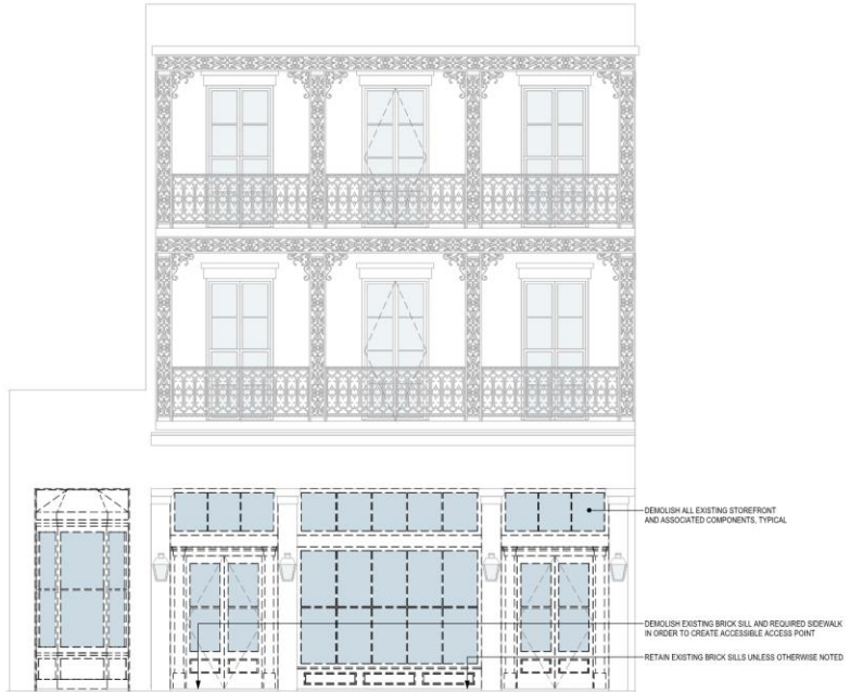
1 EXISTING & DEMOLITION BOURBON STREET ELEVATION 1/4" = 1'-0"
