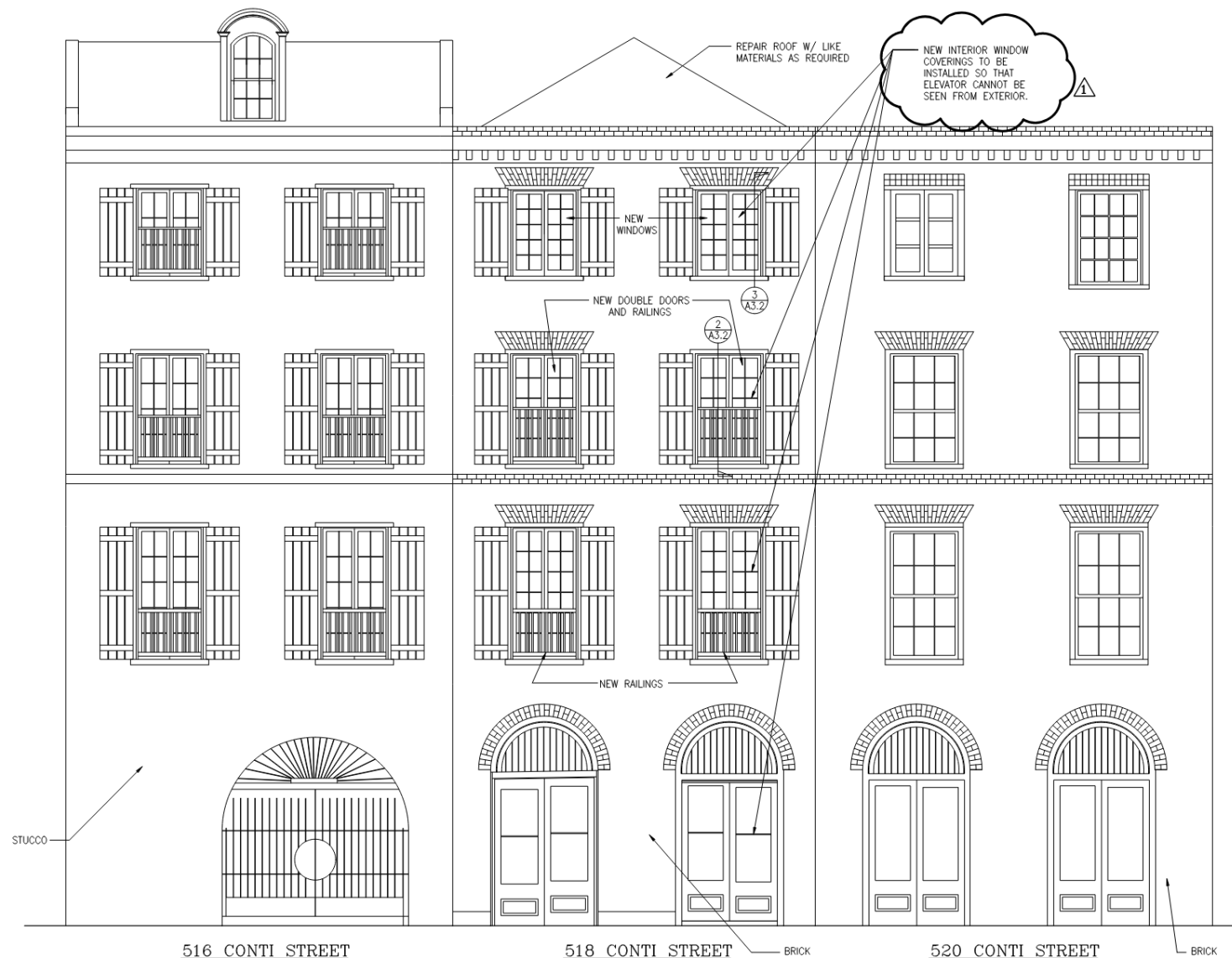
1 PROPOSED NEW CONTI STREET ELEVATION SCALE: 1/4"=1'-0"
