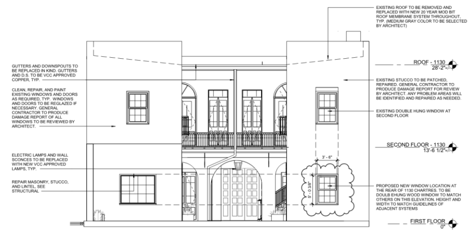
1 REAR ELEVATION - 1130 CHARTRES VCC-3 3/16" = 1'-0"
