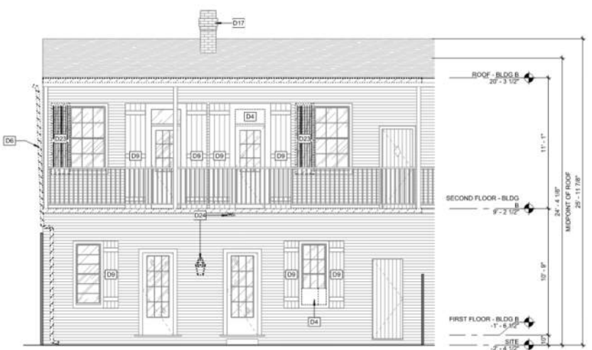
1 NORTH EXTERIOR ELEVATION BUILDING B - DEMOLITION ANSI 1/4" = 1'-0"
