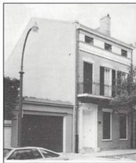
Virginia McAlester's Example of Greek Revival Townhouse in New Orleans Greek Revival Frieze Band Windows with stepped/square and dentil trim elements
