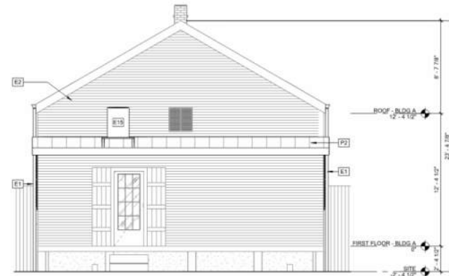
3 SOUTH EXTERIOR ELEVATION 1/4" = 1'-0"
