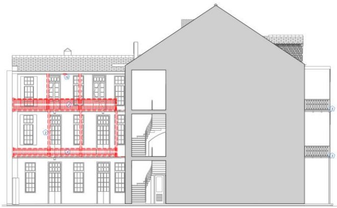
3 | COURTYARD ELEVATION - EAST - DEMO 1/8" = 1'-0"
