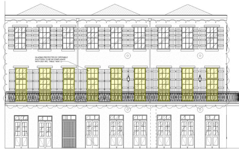
VCC EAST ELEVATION - BOURBON ST. (2) 1/8" = 1'-0"
