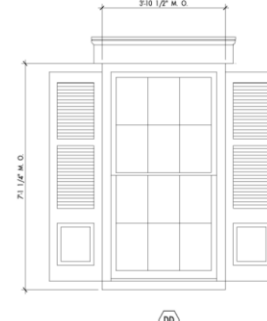
DD REPAIRED EXISTING DOUBLEHUNG WINDOWS AT MAIN STRUCTURE
