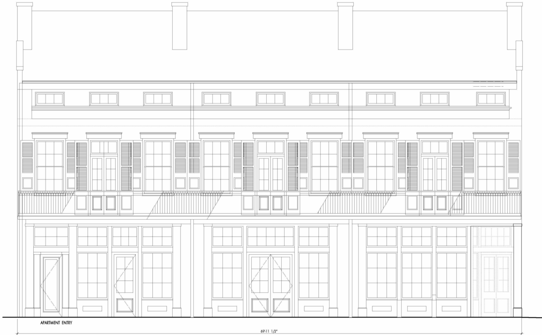
1 PROPOSED ELEVATION TO DAUPHINE STREET 1/4" = 1'-0"
