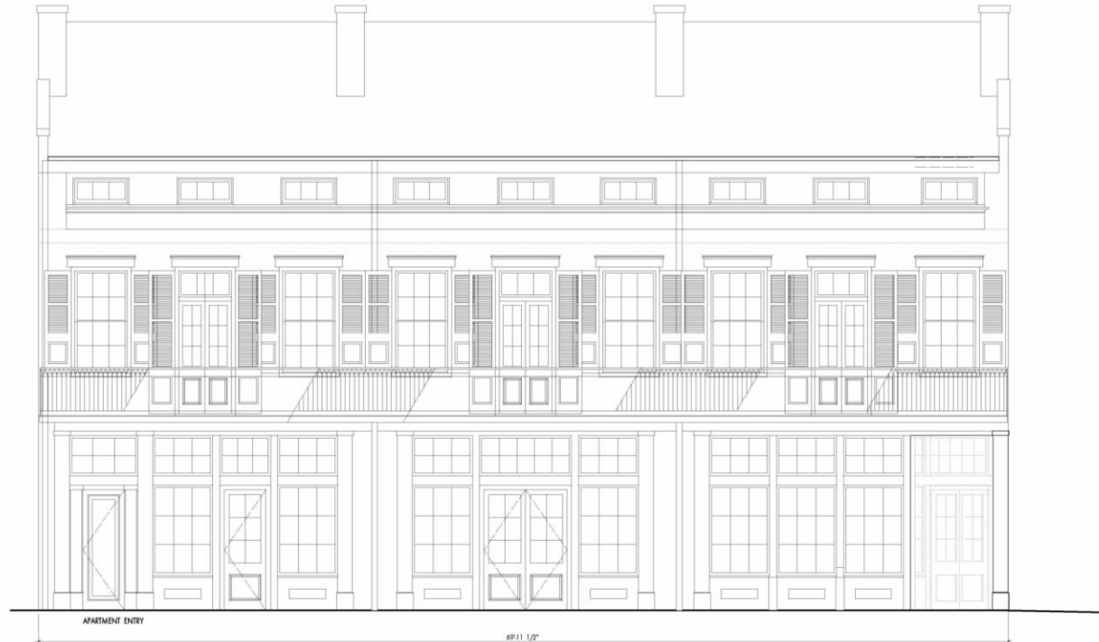
1 PROPOSED ELEVATION TO DAUPHINE STREET 1/4" = 1'-0"
