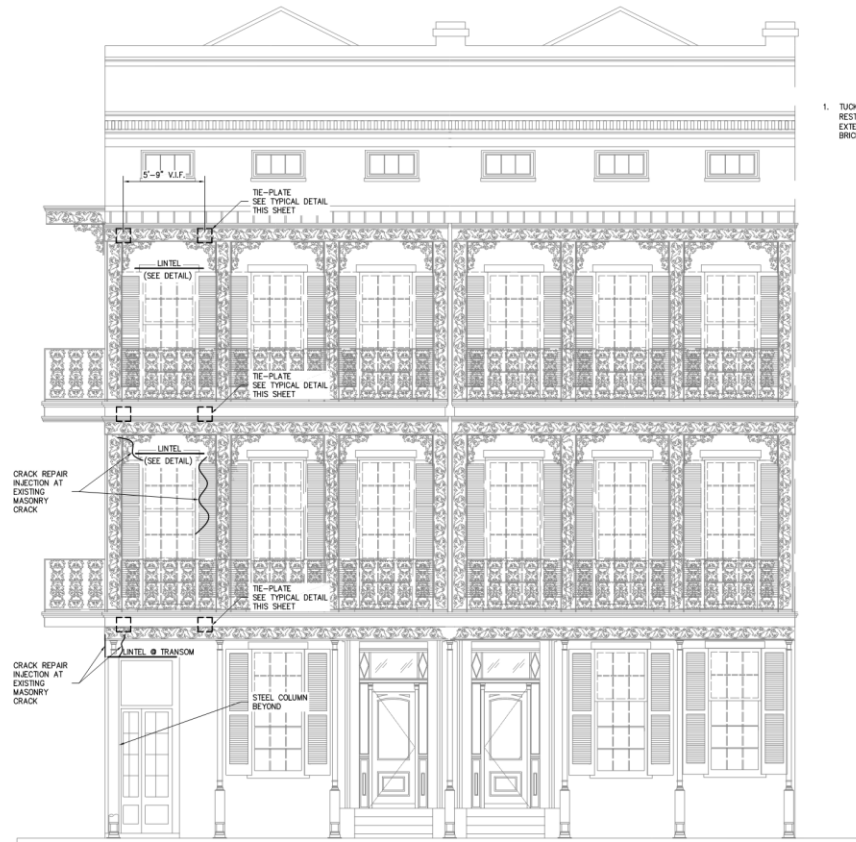
FRONT ELEVATION (RAMPART STREET) SCALE: 1/4"=1'-0"
