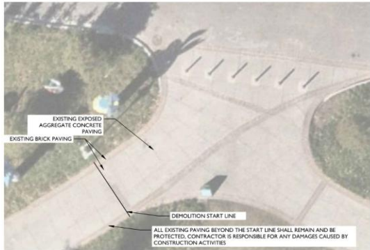
3 EXISTING PATH DEMOLITION Scale: NTS
