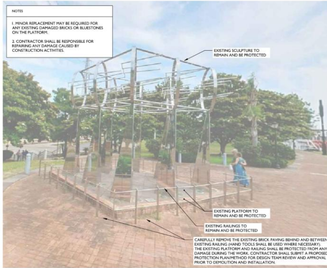
4 EXISTING SCULPTURE WITH BRICK PLATFORM AND RAILING TO REMAIN AND BE PROTECTED Scale: NTS
