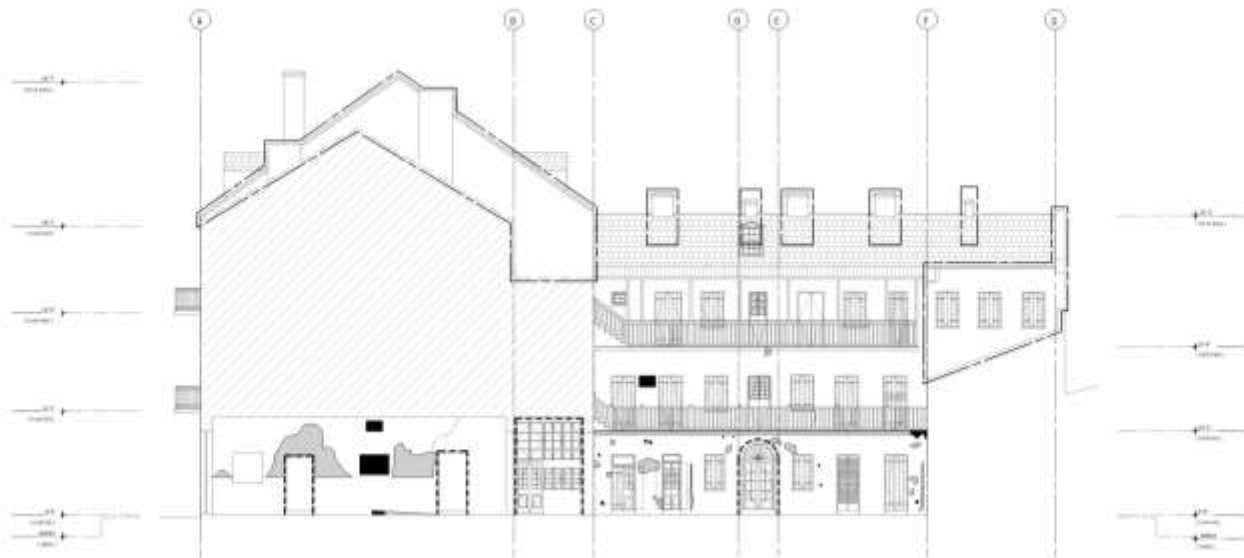
1 EAST ELEVATION - EXTERIOR WALL CONDITION SCALE: 1/8" = 1'-0"
