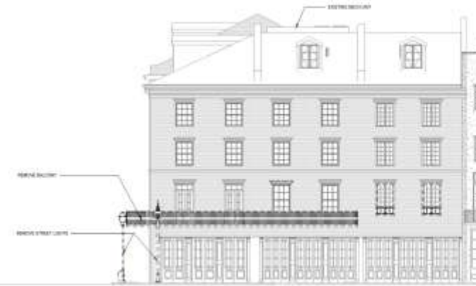
DEMOLITION DECATUR STREET 18' x 12'
