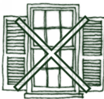
The louvered shutters are the incorrect size for the window
