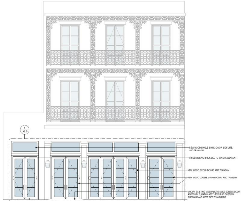
2 PROPOSED BOURBON STREET ELEVATION 1/4" = 1'-0"
