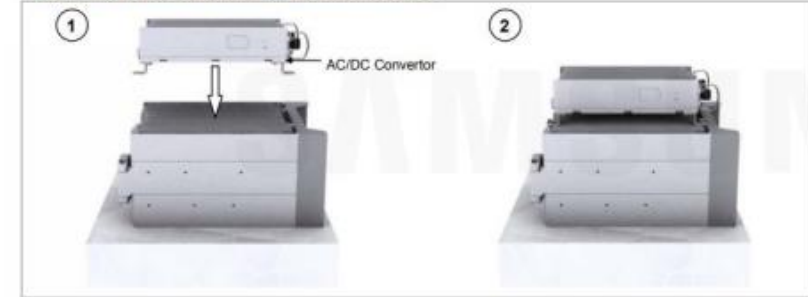
Figure 17. Fixing AC/DC Converter_Front Installation (1)
