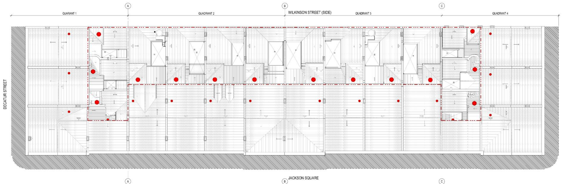
1 OVERALL ROOF PLAN - EXHAUST LOCATIONS CC1.00 SCALE: 1/16" = 1'-0"
