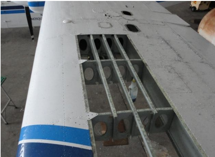
Figure 14. Wing skins removed for corrosion repairs.
