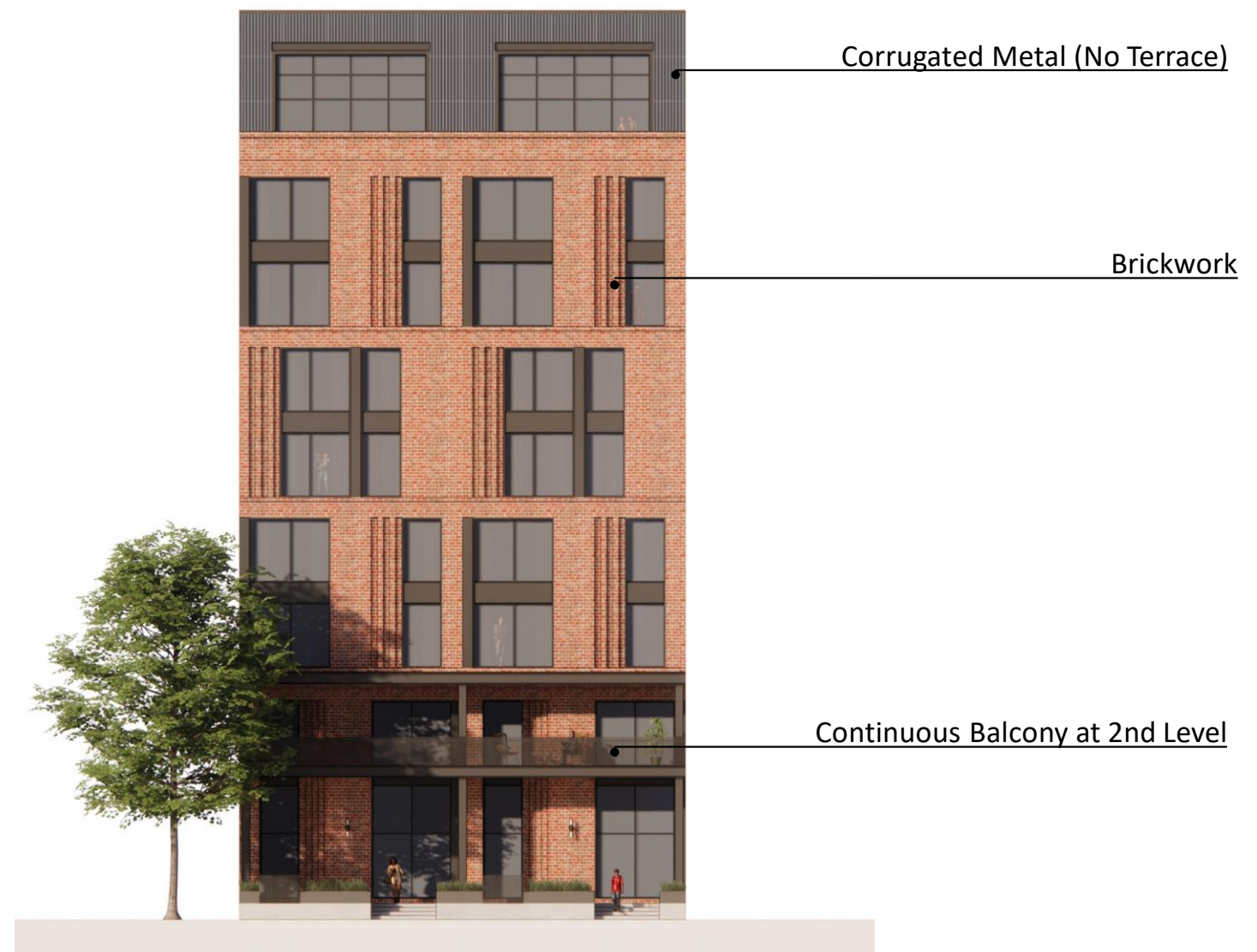
B. Race Street Facade 7-9 levels; all residential
