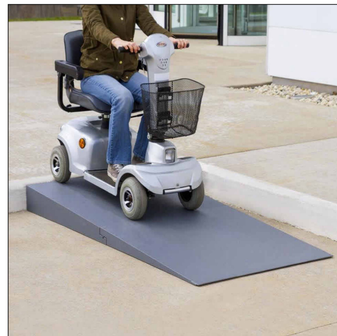
4) FOAM ADA RAMP • MAX 1/12 SLOPE FROM ADA PLATFORM TO STREET GRADE MIN. 3' WIDTH
