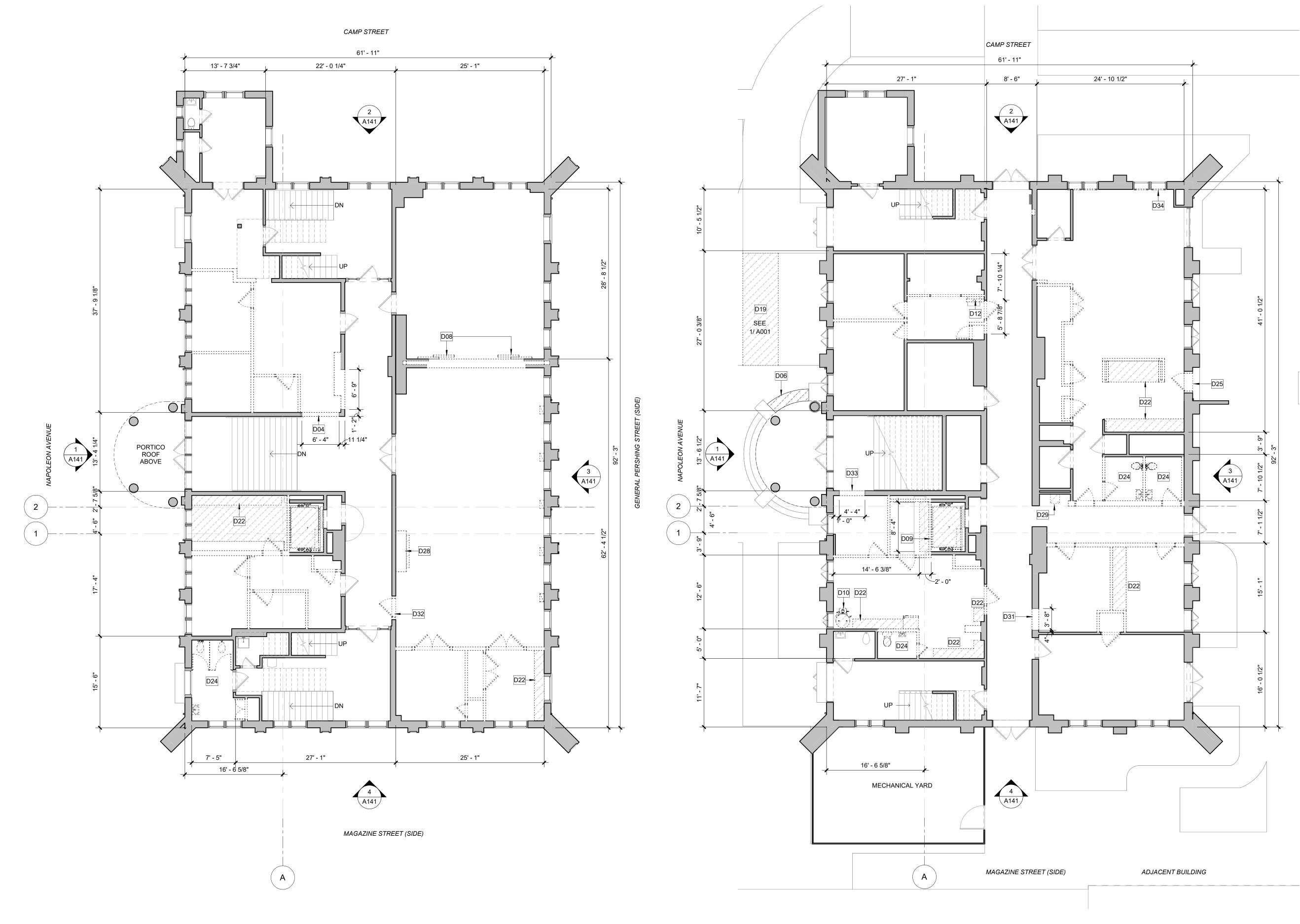
2 SECOND FLOOR PLAN - DEMOLITION A101 1/8" = 1'-0"
