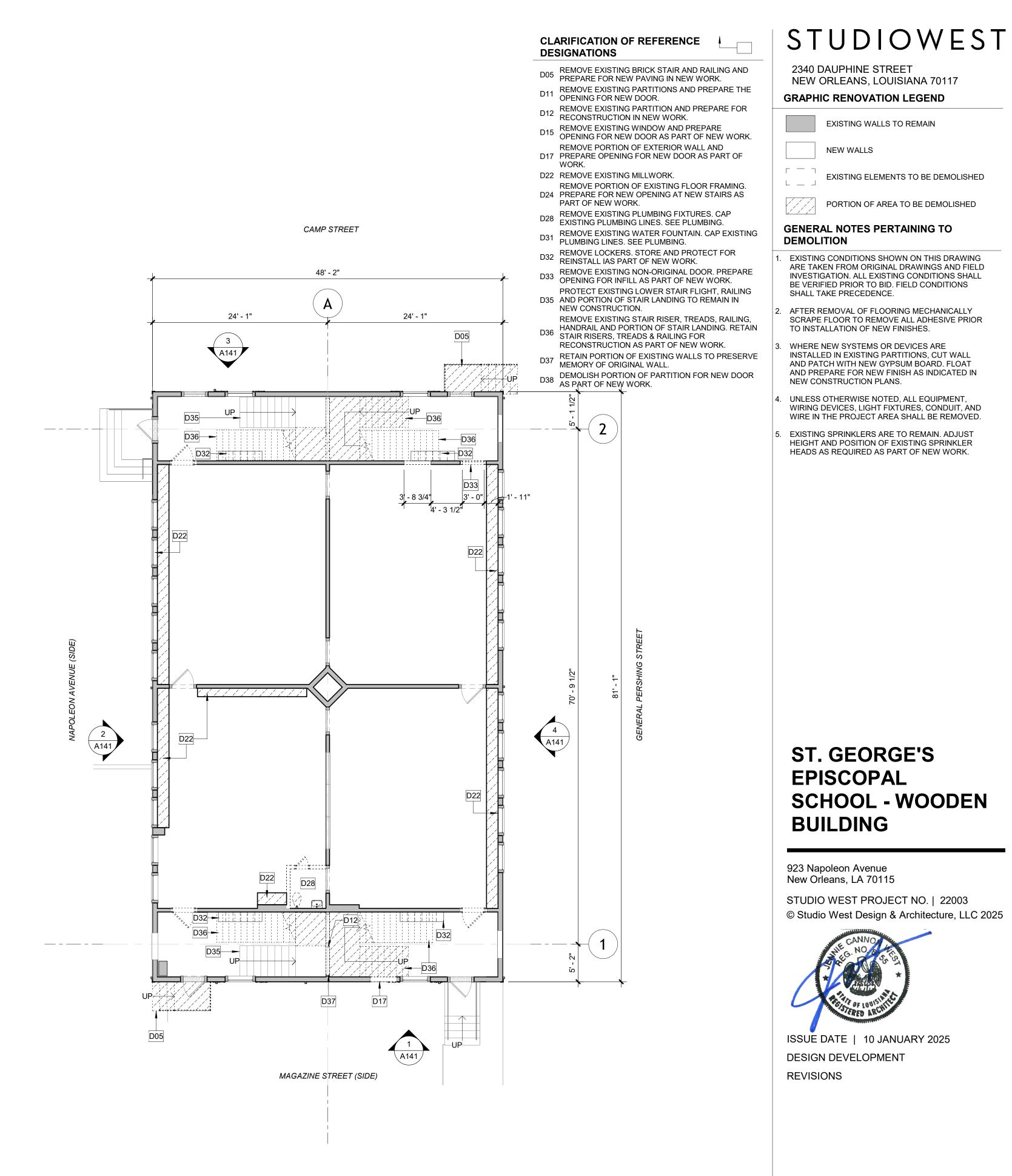
2 SECOND FLOOR PLAN - DEMOLITION A101 1/8" = 1'-0"
