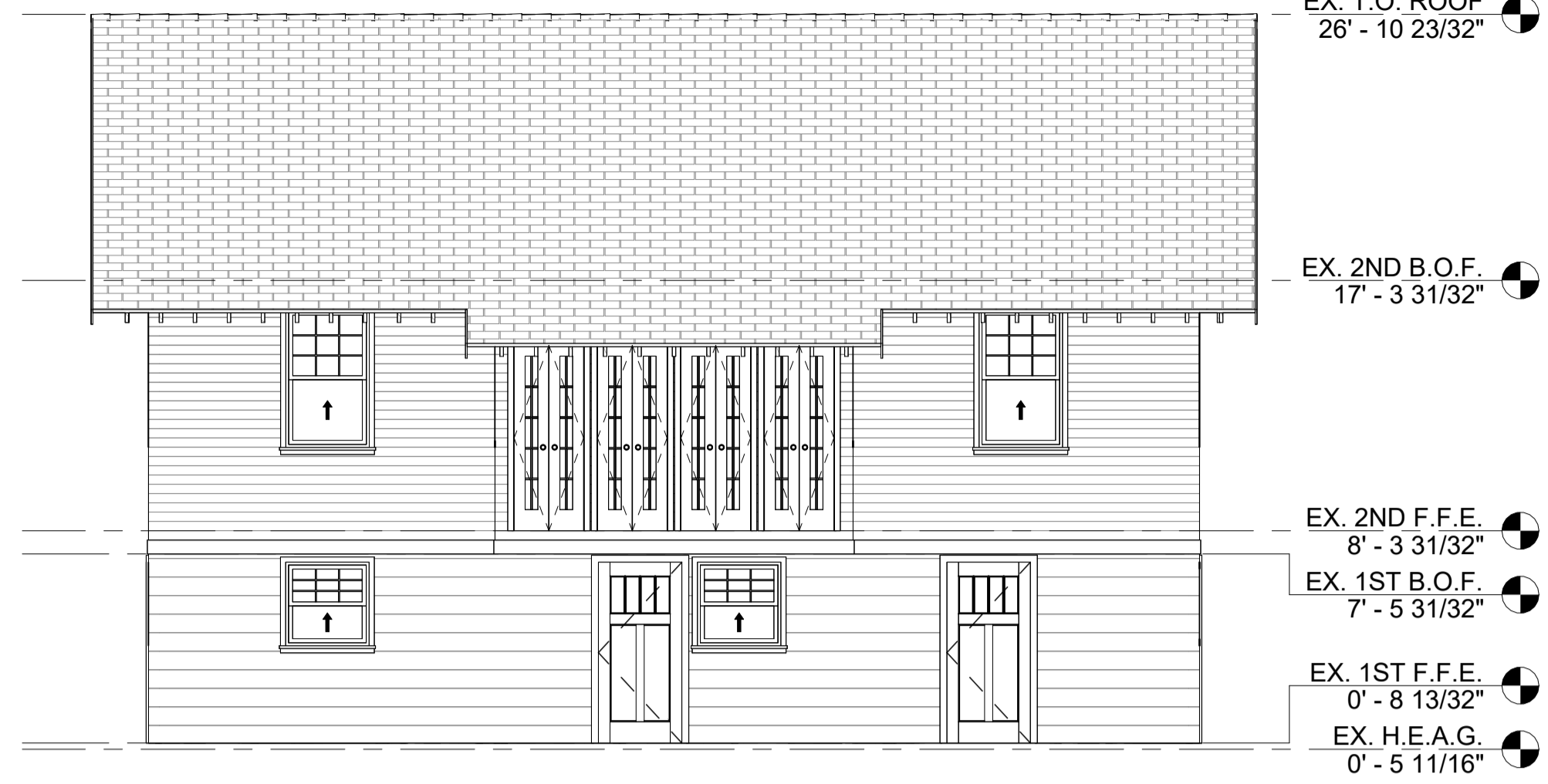
4 EXISTING REAR ELEVATION 3/16" = 1'-0"
