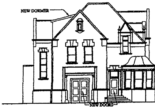
ST. PHILIP STREET FRONT ELEVATION SC: 1/16" = 1'-0"
