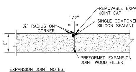
1. PREFORMED EXPANSION JOINT WOOD FILLER AND SINGLE COMPONENT SILICON SEALANT SHALL CONFORM TO SECTION 1005 JOINT MATERIALS FOR PAVEMENTS AND STRUCTURES" OF THE LOUISIANA DEPARTMENT OF TRANSPORTATION STANDARD SPECIFICATIONS.
