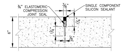
LONGITUDINAL JOINT NOTES: 1. LONGITUDINAL JOINTS SHALL BE SAWCUT AS SHOWN, FILLED WITH PREFORMED ELASTOMERIC COMPRESSION JOINT SEALS, AND SEALED WITH SINGLE COMPONENT SILICON SEALANT. JOINT SEALS AND SILICON SEALANT SHALL CONFORM TO SECTION 1005 "JOINT MATERIALS FOR PAVEMENTS AND STRUCTURES" OF THE LOUISIANA DEPARTMENT OF TRANSPORTATION STANDARD SPECIFICATIONS.
