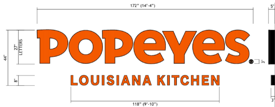
④ ILLUMINATED CHANNEL LETTERS (FRONT VIEW) N.T.S.
