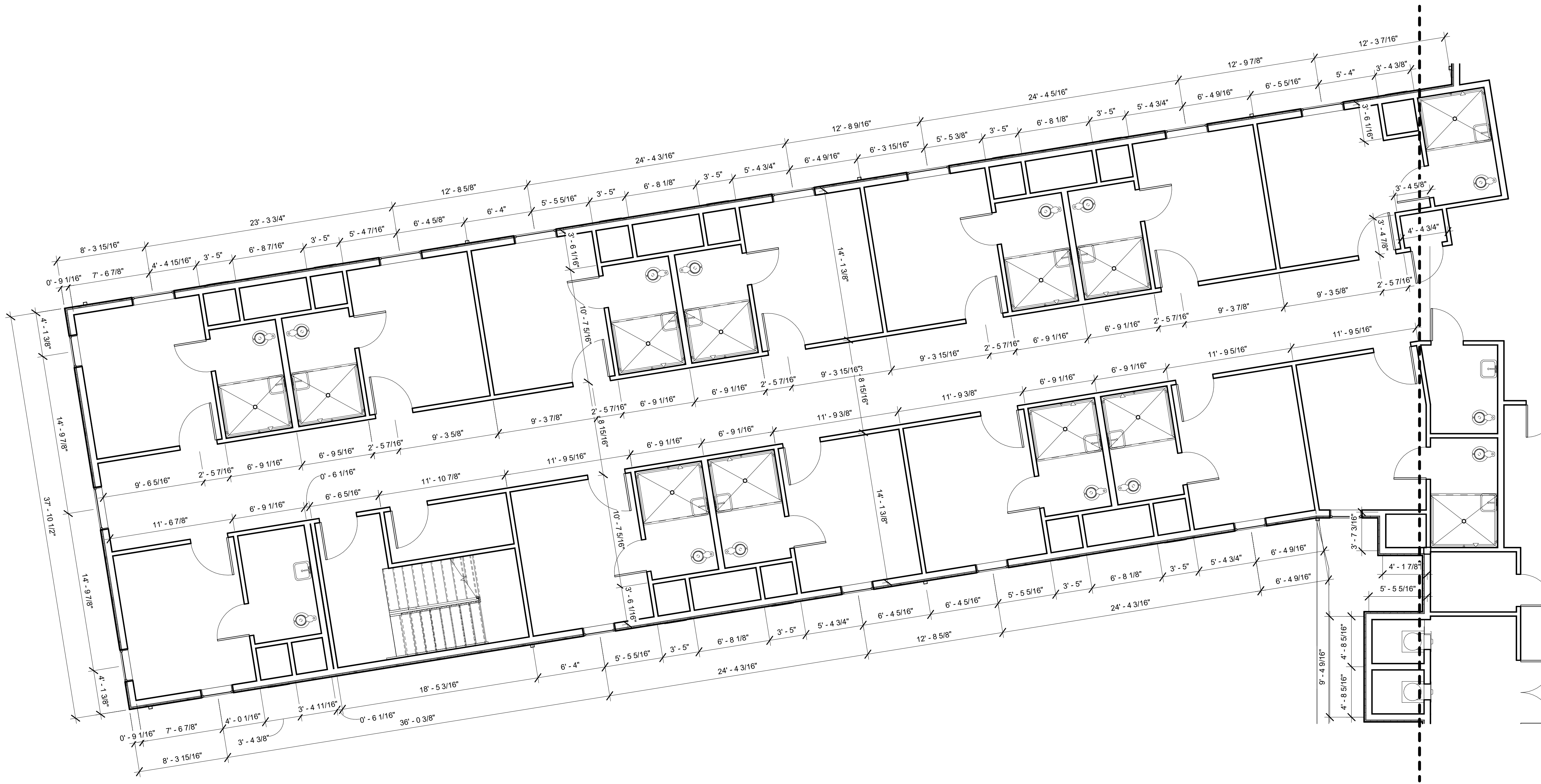
SECOND FLOOR DIMENSIONAL PLAN - Enlarged Plan D 3/16" = 1'-0"
