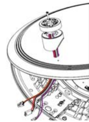
7-Pin receptacle placement
