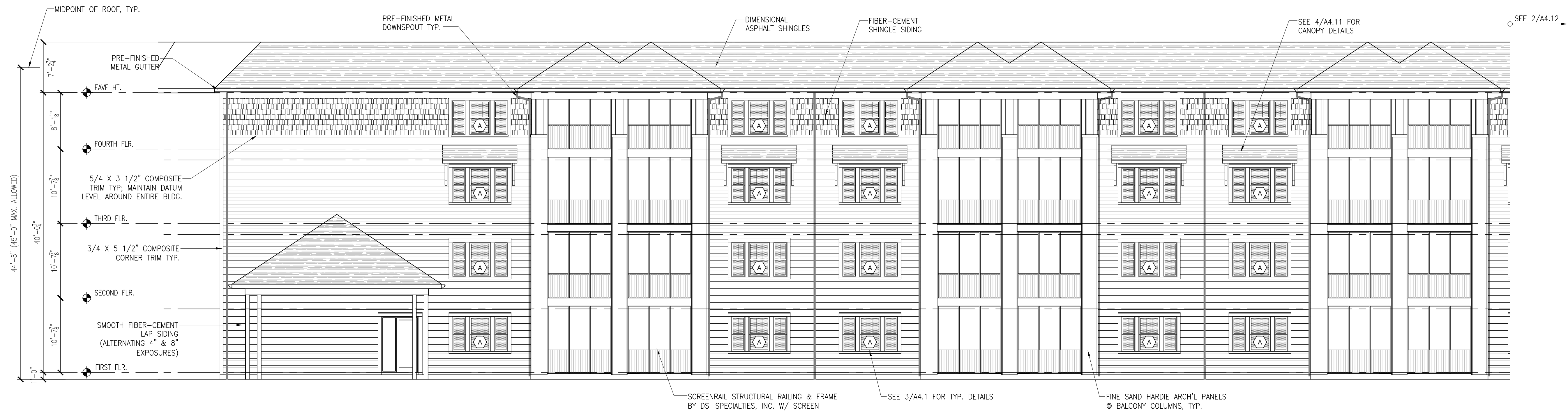
1 PARTIAL REAR ELEVATION – BLDG. H A4.12 1/8" = 1' - 0"
