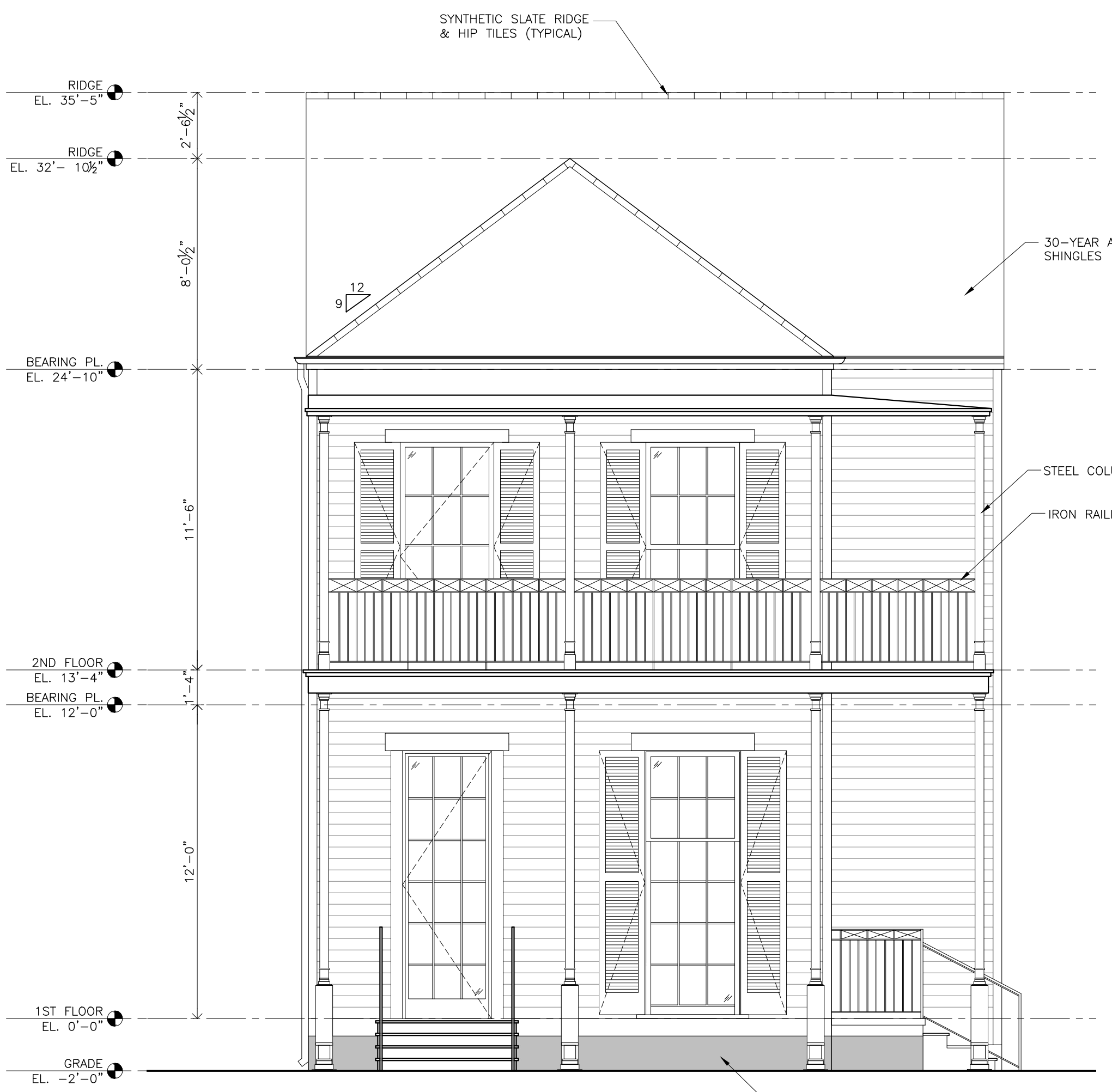
1 FRONT ELEVATION (CANAL STREET) SCALE: 1/4" = 1'-0"
