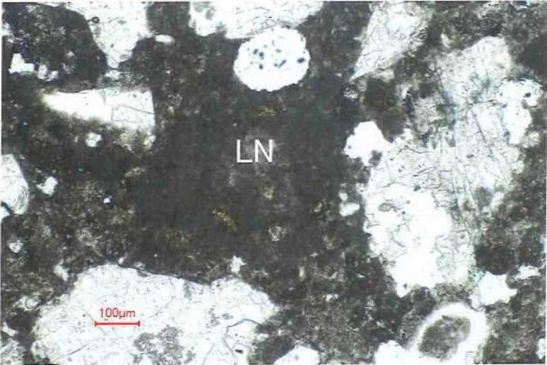
SAMPLE ID: 215-225 MAG: 100x DESCRIPTION: Sand-sized lime nodule (LN) within mortar binder in thin section under transmitted plane polarized light.
