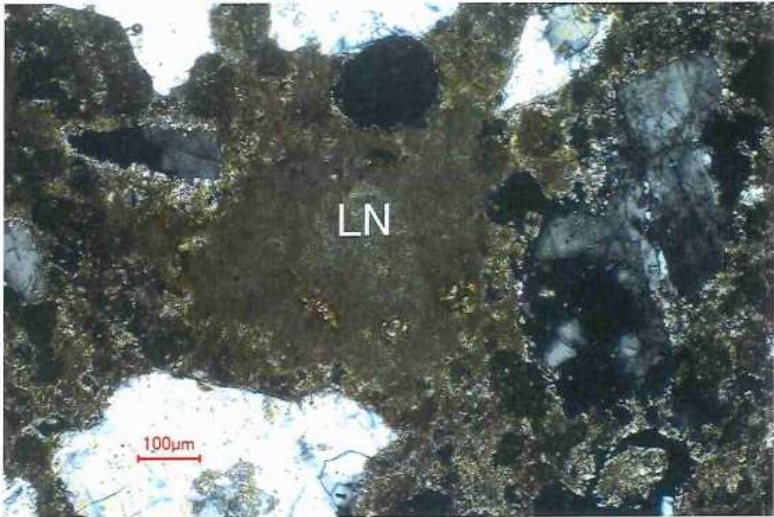
SAMPLE ID: 215-225 MAG: 100x DESCRIPTION: Same view as above under transmitted cross polarized light. Note the fully carbonated (brightly-colored) binder and small portion of non-carbonated 'core' or center of nodule.
