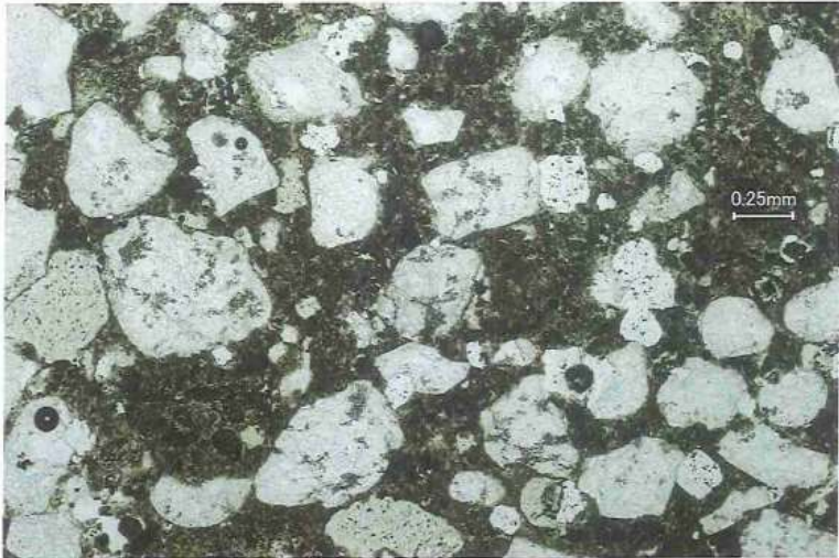
SAMPLE ID: 215-225 MAG: 40x DESCRIPTION: Overall view of mortar sample in thin section under transmitted plane polarized light.
