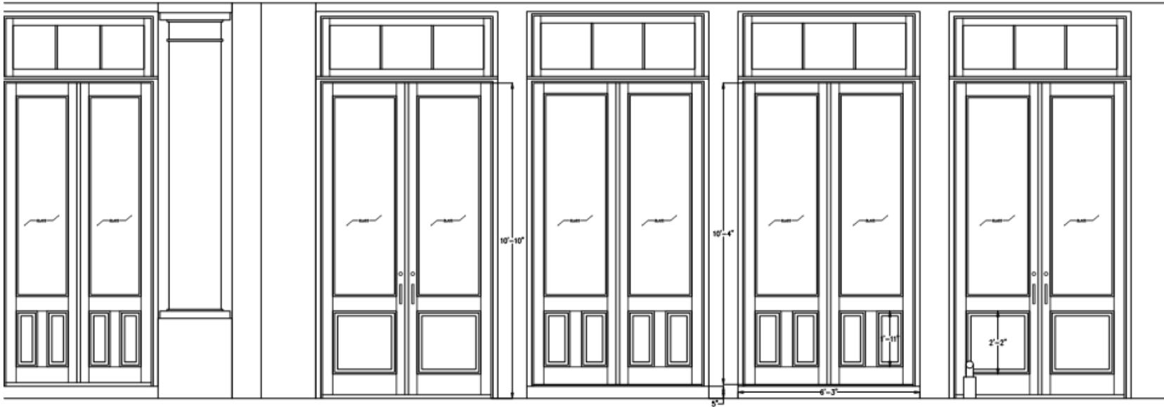
4 Chartres St. Elevation (proposed changes) Scale: 1/4" = 1'-0"
