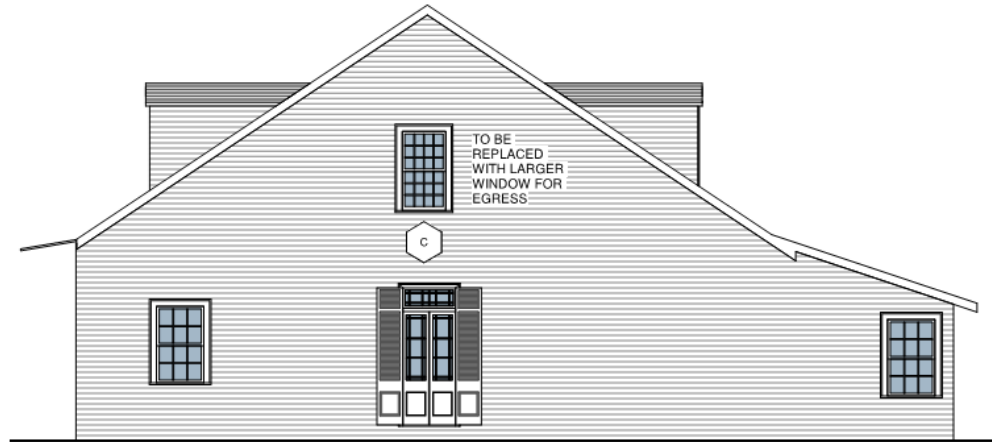
7 PROPOSED ELEVATION - SIDE - BARRACKS ST. 1/8" = 1'-0"
