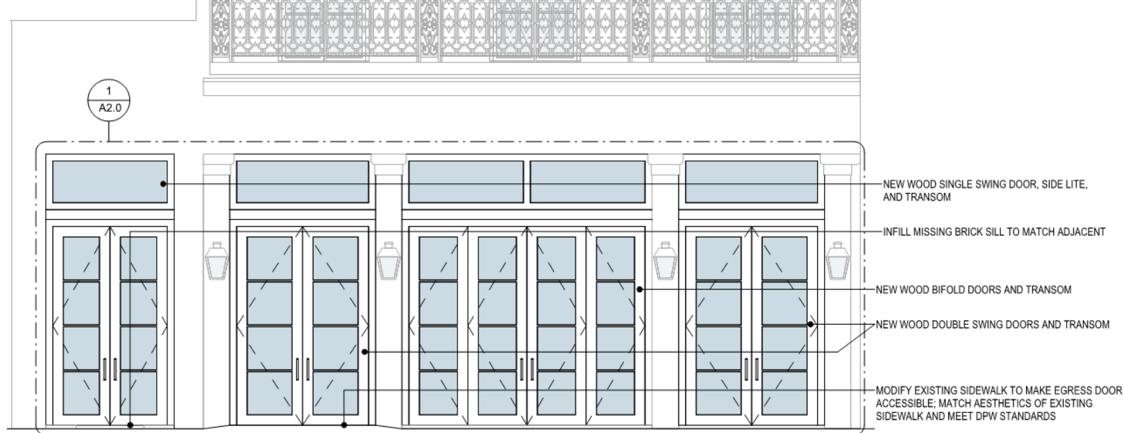
② PROPOSED BOURBON STREET ELEVATION 1/4" = 1'-0"
