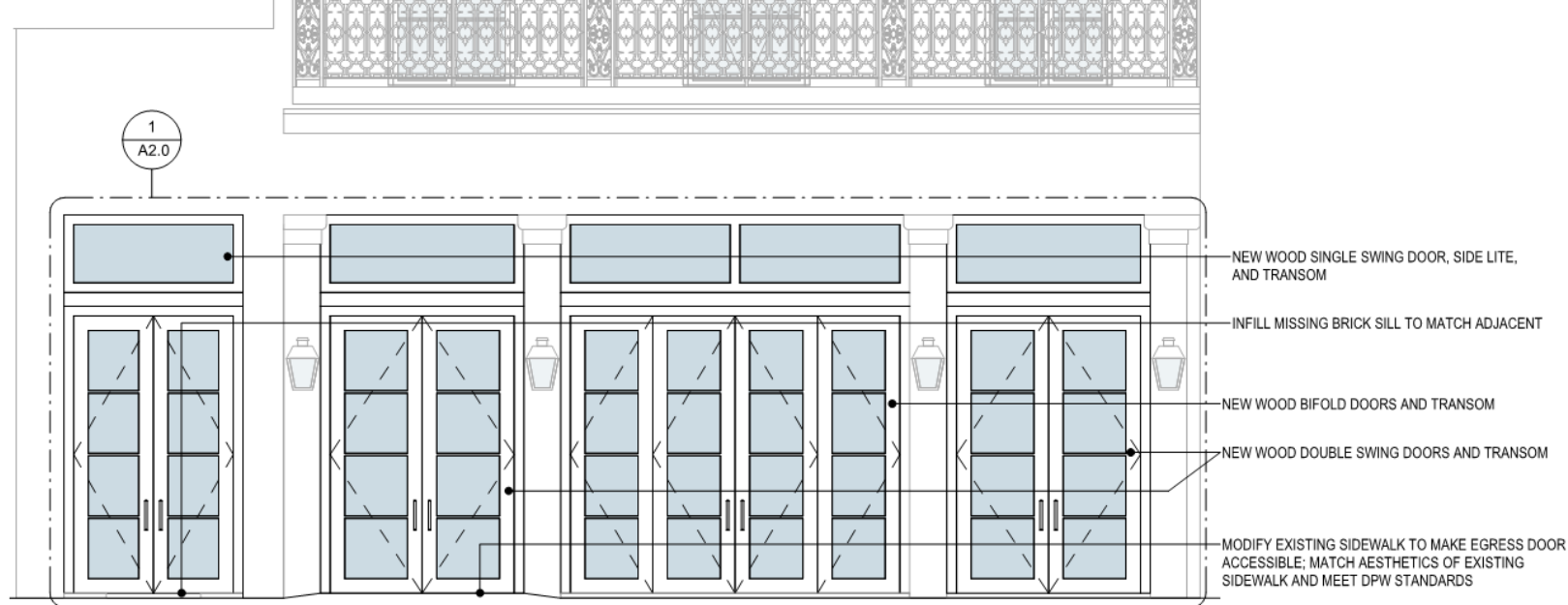
② PROPOSED BOURBON STREET ELEVATION 1/4" = 1'-0"
