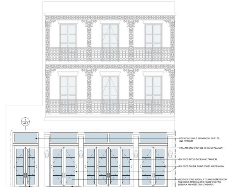
2 PROPOSED BOURBON STREET ELEVATION 1/4" = 1'-0"
