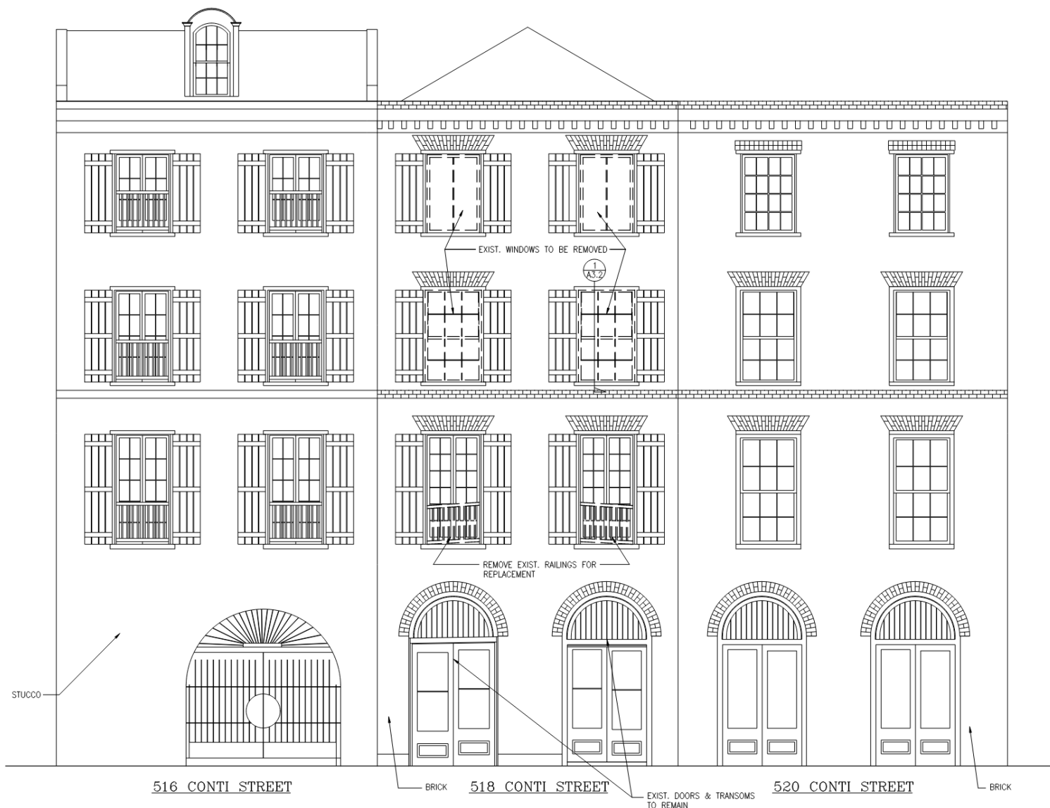
1 EXISTING/DEMOLITION CONTI STREET ELEVATION SCALE: 1/4"=1'-0"
