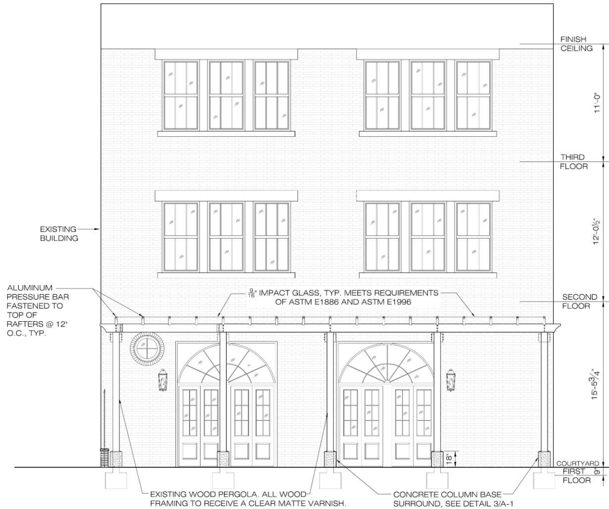
2 Pergola Elevation @ Courtyard A-1 3/16" = 1'-0"
