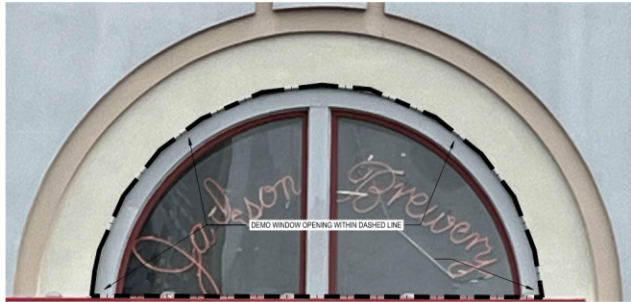
3 EXTERIOR DEMO MATERIAL LIMITS A2.07 NO SCALE
