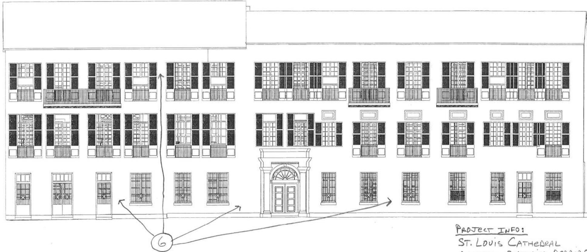
⑥ PREP + PAINT. STRIP ELASTOMERIC PAINT FROM BUILDING USING SMART STRIP PRO. PRESSURE WASH AND HAND SCRAPE TO GET TO PAINTABLE SURFACE. PATCH CRACKS AS NEEDED. PRIME WITH BENJAMIN MOORE ULTRA SPEC EXT. LATEX PRIMER. PAINT TWO COATS WITH BENJAMIN MOORE AURA WATERBORNE EXTERIOR FLAT N629.
