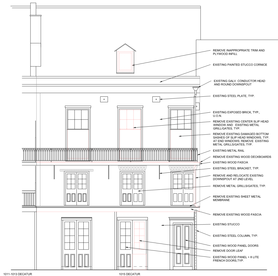
EXISTING / DEMOLITION FRONT ELEVATION SC: 1/4" = 1'-0"
