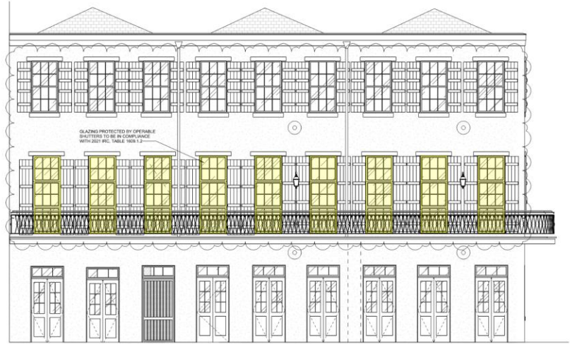
VCC EAST ELEVATION - BOURBON ST. (2) 1/8\"/>
