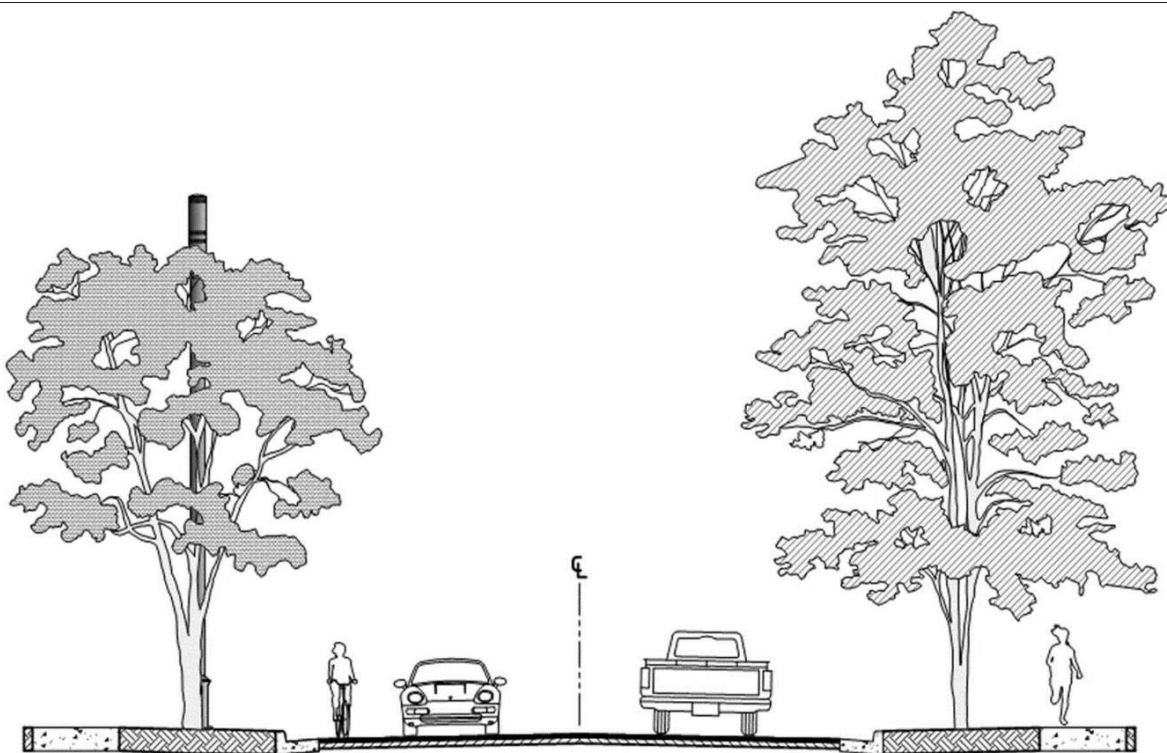
Figure 5-3.1: Freestanding Small Cell in Public Right-of-Way
