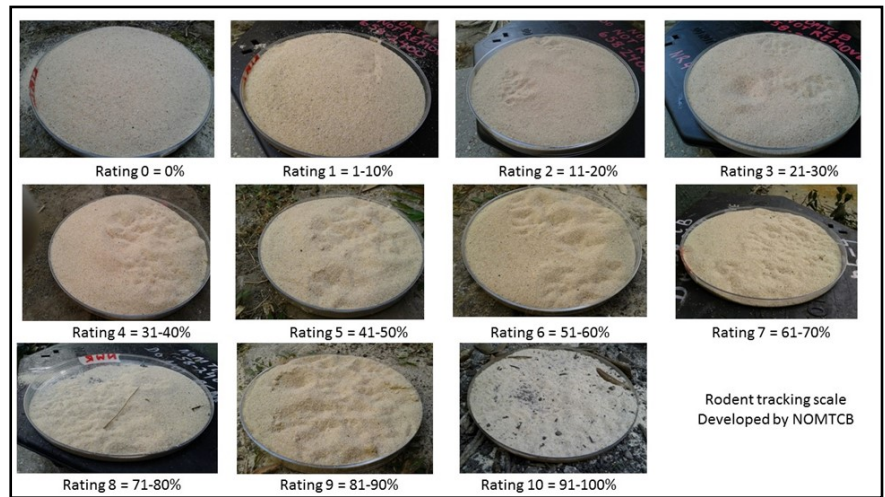
Figure 14. Rodent tracking scale developed by Friederike Bauder, Philip L. Smith and Claudia Riegel. This scoring method was incorporated into efficacy trials in order to be more precise with rodent activity at a site.
