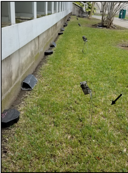
Figure 13. Game cameras were used to quantify rodent activity in rodenticide efficacy trials.
