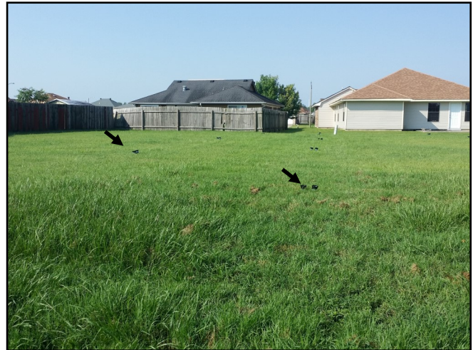
Figure 9. First field trial to assess larvicide deposition of the off the shelf configuration of the Buffalo Turbine.. Arrows indicate collection cups placed at 20' intervals for 100'.
