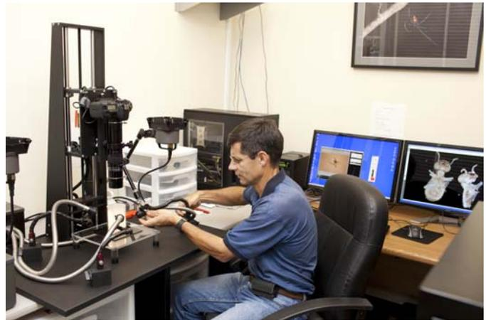
**Figure 28.** Ed Freytag sets up the fiber optic flashes of the Visionary Digital microscope.
