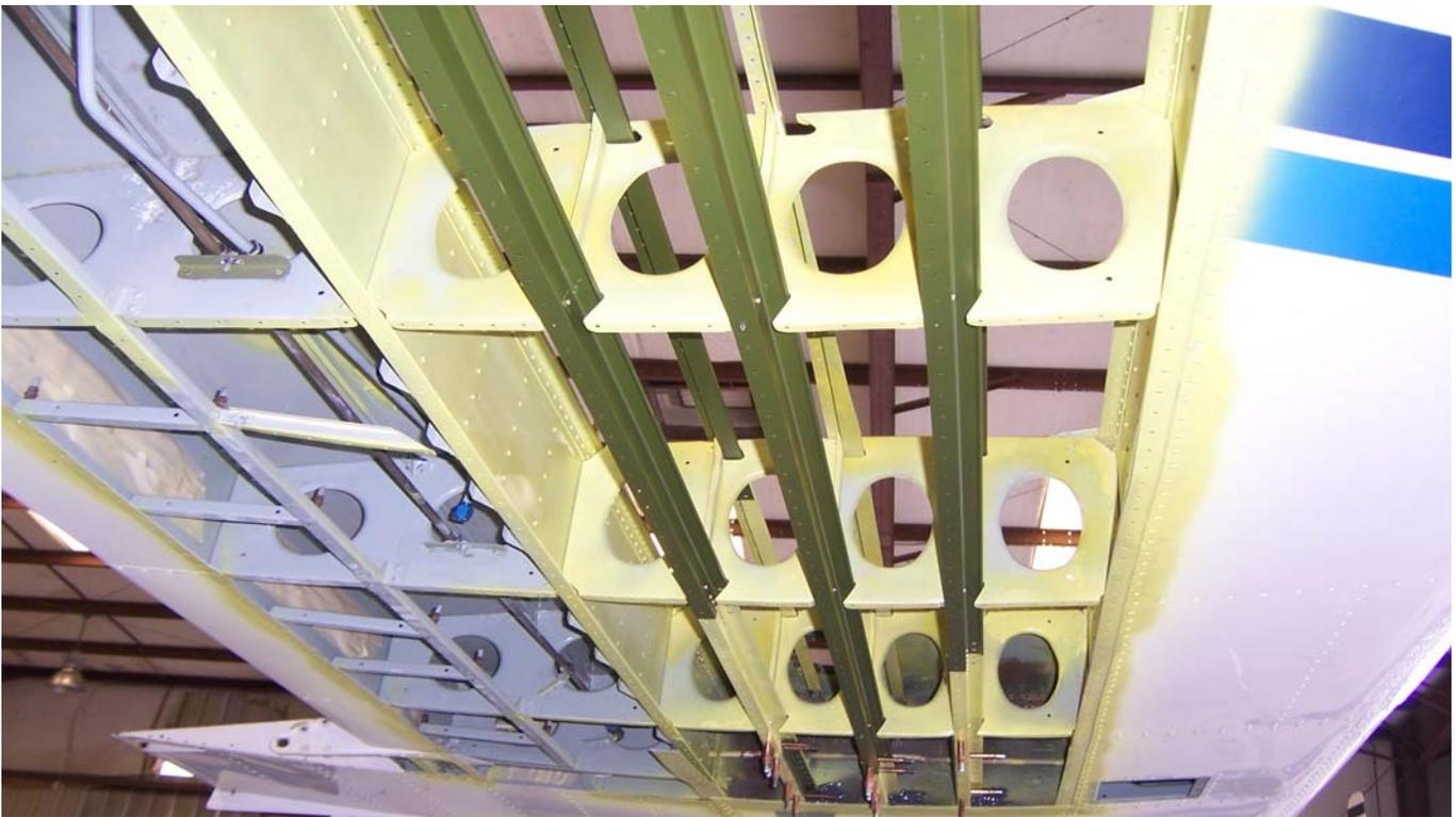
**Figure 21.** The right wing of the Britten-Norman Islander after remediation of corrosion.
