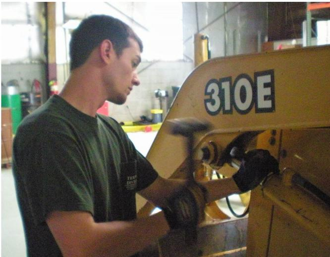
Figure 25. Mr. Bryan Wirth removes a hydraulic cylinder from a backhoe for cleaning and repair.
