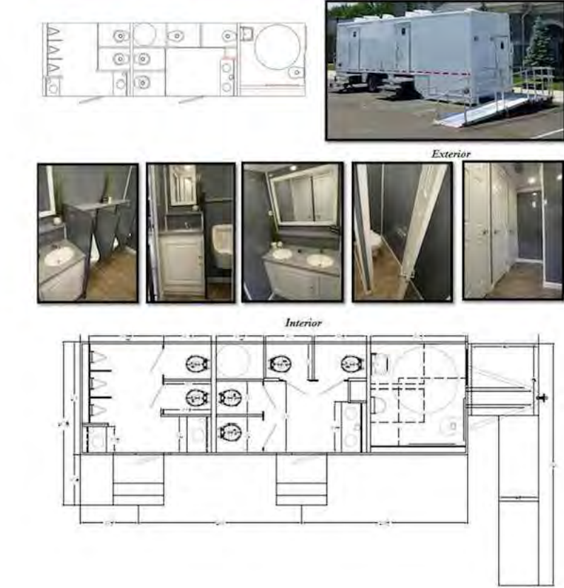
4 TEMPORARY BATHROOM DETAILS NOT TO SCALE
