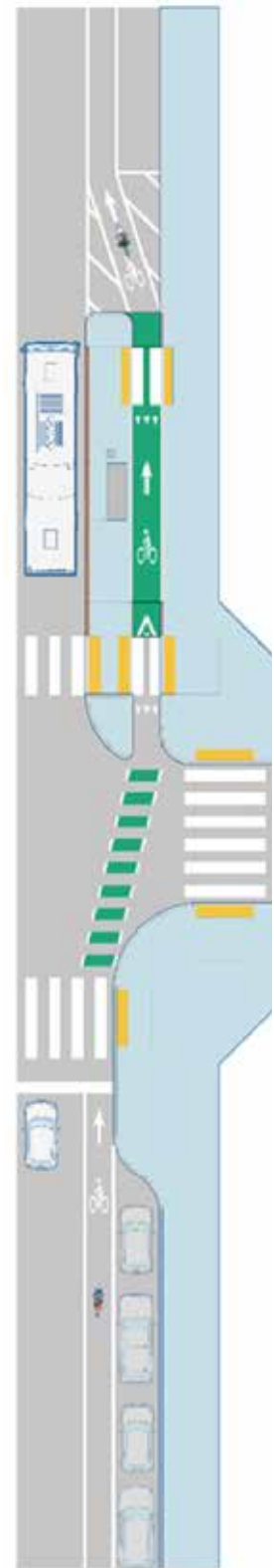
FIGURE 14 Curb Extension Design A floating bus stop and separated bike lane barrier can function as curb extensions—either as separate or joint facilities.
