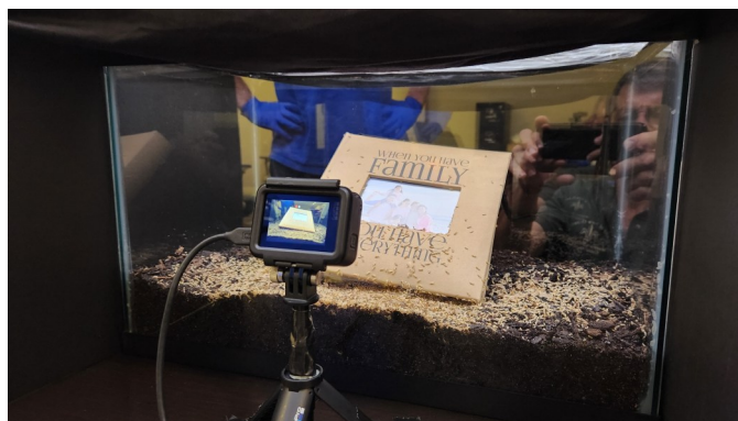
Figure 37. Setup for taking time-lapse photos of Formosan termites eating the item in the aquarium..
