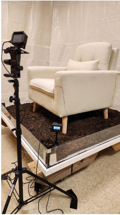
Figure 38. The “Megatank” setup with chair, soil, termites, and GoPro cameras.
