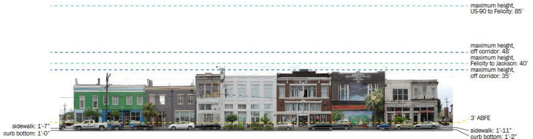
Elevation of curb bottom, sidewalk, and required 3' building height, on O.C. Haley Blvd. as well as zoning height limitations Source: Elevation survey, conducted by MSMM, 2015; City Comprehensive Zoning Ordinance, 2015
