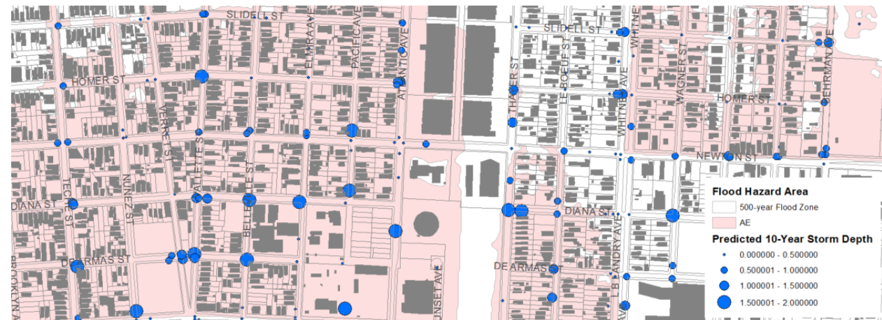
Newton St. flood hazards and drainage infrastructure deficiencies
