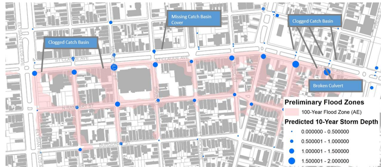
St. Claude Ave. flood hazards and drainage infrastructure deficiencies
