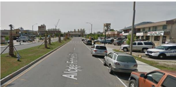
Existing number of travel lanes exceed traffic demand. Converting one lane to parking would create about 12 parking spaces mitigating redesign of public space along the sidewalk
