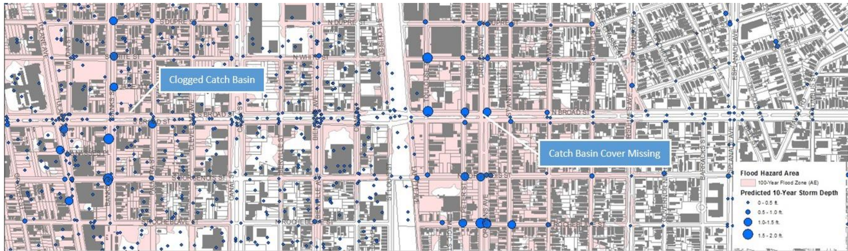
Broad St. flood hazards and drainage infrastructure deficiencies
